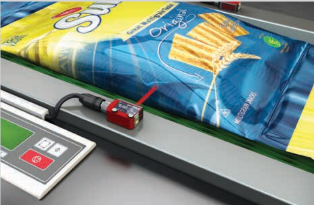
Content check with radiation through films
